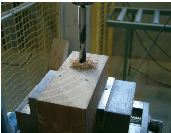
Figure 2: Taking a sample core
